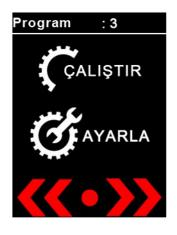
The touchpad-screen of the step control device is touch-sensitive. This main screen appears shortly after the kiln is turned on.
