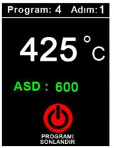
This screen appears if the step time has elapsed but the preset end temperature has not been reached.
