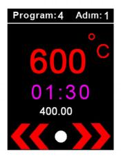
We can check the step values and proceed to the next settings screen by tapping the ">>" sign at the bottom.
